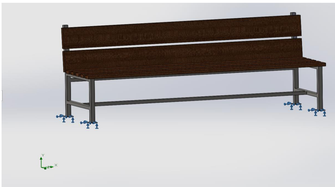
Figure 13: adding fixture geometry
